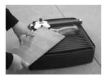
• Push the angle guide (B) together with the tile to be cut towards the diamond wheel (H).
